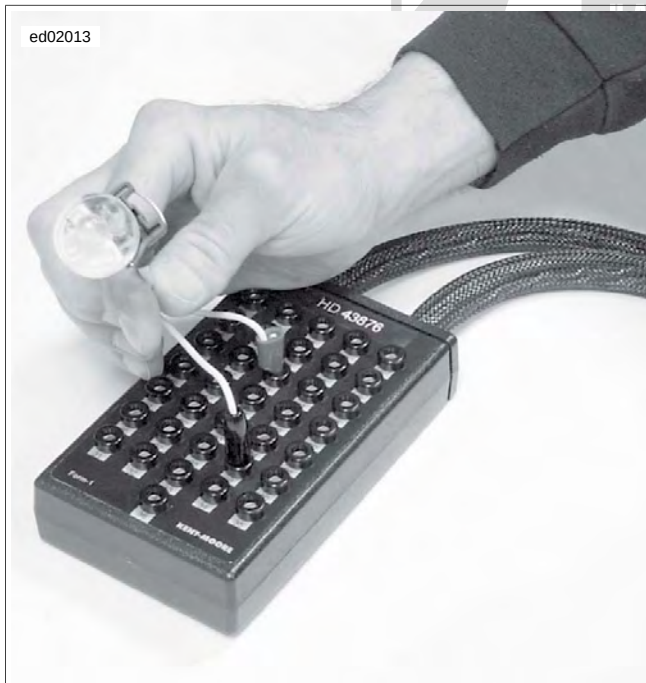
Figure 6-43. Ignition Coil Circuit Test
