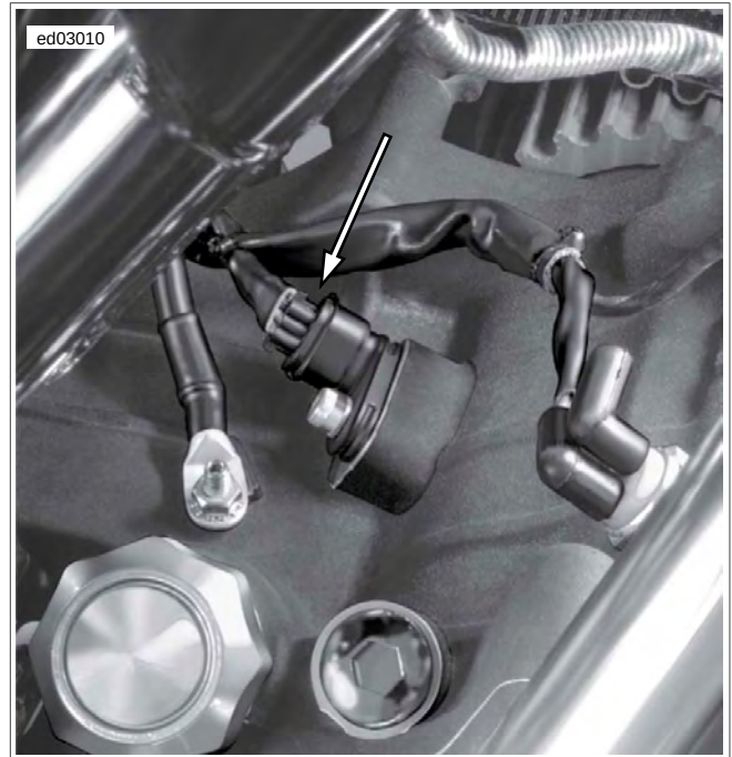
Figure 6-17. VSS Location (Under Starter)
