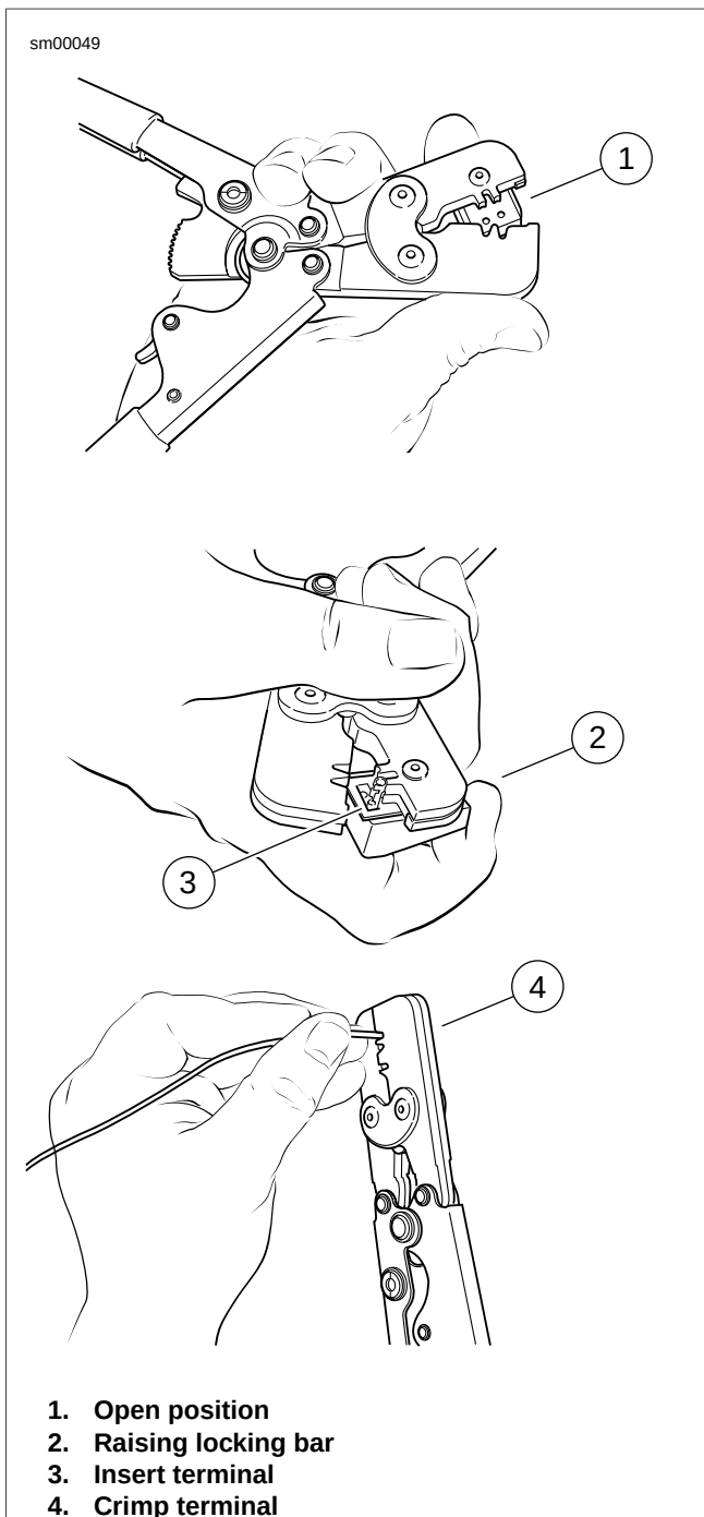
Figure A-19. Delphi Micro-64 Sealed Connector: Terminal in Crimper
