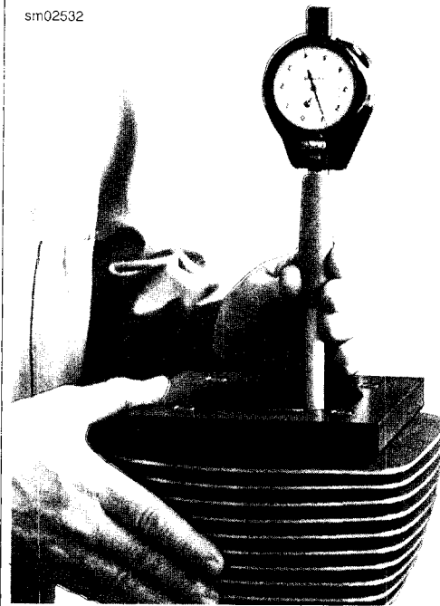
Figure 3-116. Measure for Out-of-Round and Taper
