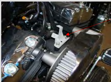
New ACR Bracket to hold wires
