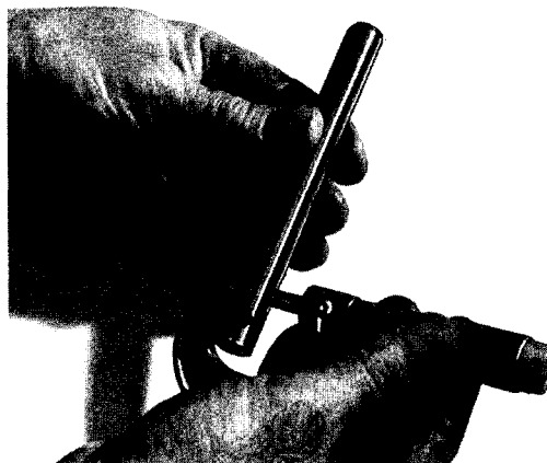
Figure 3-90. Checking Shaft to Bushing Fit
