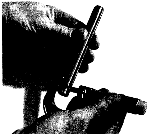
Figure 3-88. Checking Shaft to Support Plate Fit
