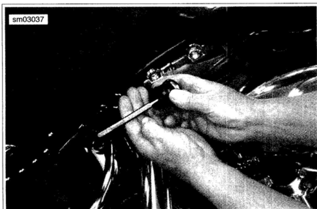
Figure 1-1. Checking Oil Tank Level
